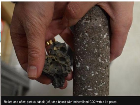
Before and after: porous basalt (left) and basalt with mineralised CO<sub>2</sub> within its pores
